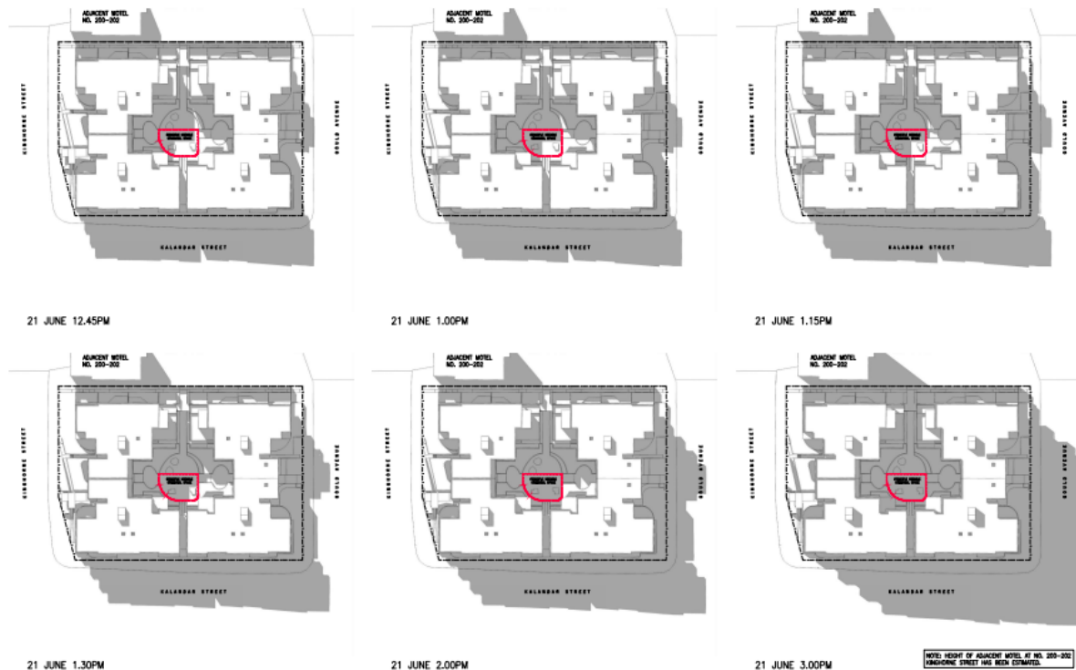
Figure 19 - Shadow diagram of the development (mid-winter) from 12:45am to 3:00pm. The proposed useable common open space indicated in red.
