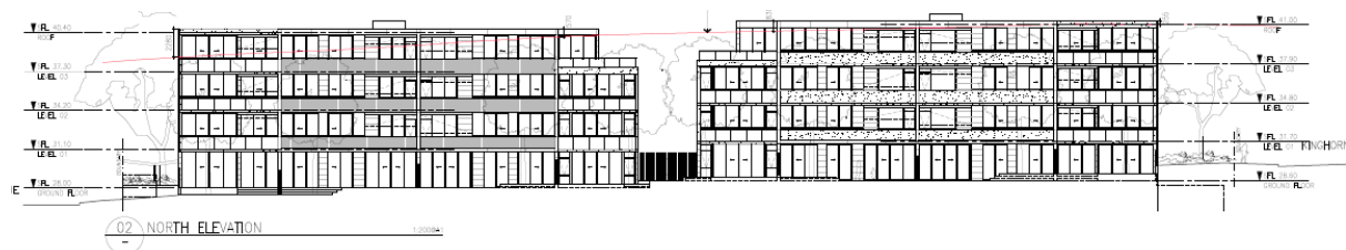
Figure 21 - Northern elevation (Kalandar Street) of the proposed development. red line indicative of the maximum height of building (11m) and the developments exceedance of the standard.
