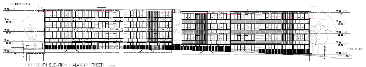
Figure 20 - Southern elevation (Kalandar Street) of the proposed development. red line indicative of the maximum height of building (11m) and the developments exceedance of the standard.
